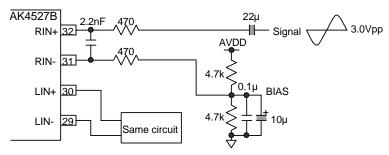
Figure 12. Single End Input Example (ADIF= "L"; Not using op-amp)
