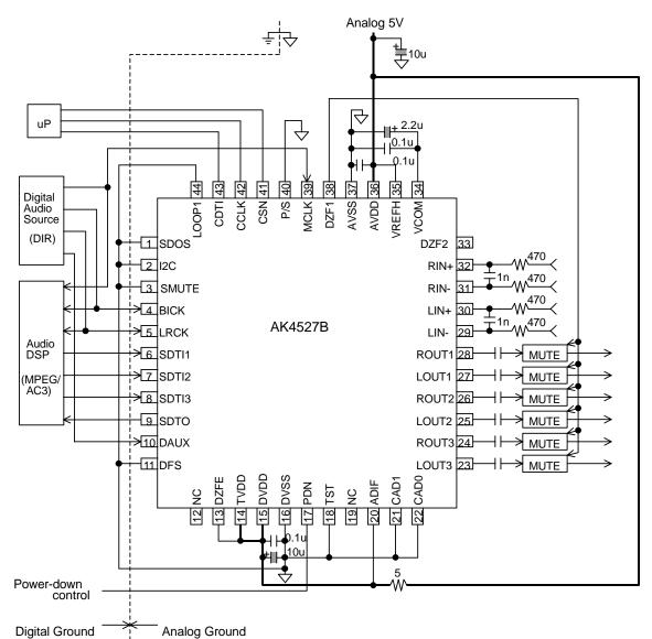
Condition: TVDD=5V, 3-wire serial control mode, CAD1-0 = "00", Full-differential input
