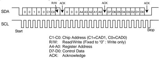
Figure 9. I<sup>2</sup>C-bus Control I/F Timing
