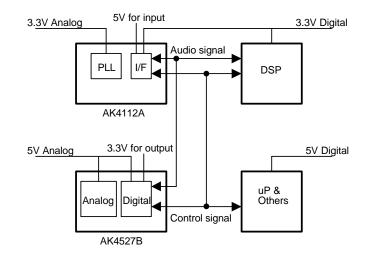
Figure 16. Power supply connection example
