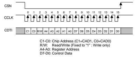
Figure 8. 3-wire Serial Control I/F Timing
