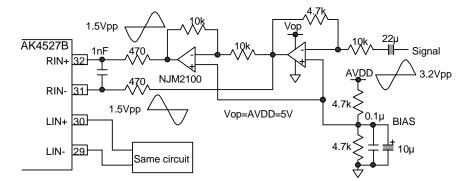
Figure 14. Differential Input Buffer Example (ADIF= "H"; Using op-amp with single power supply)
